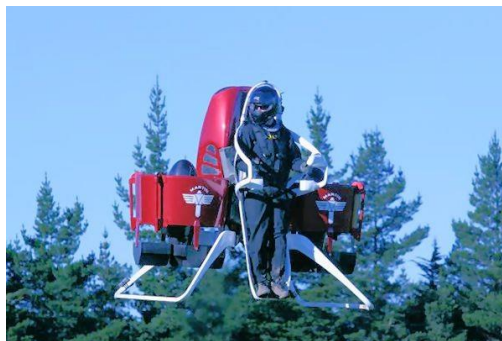
14.90 The P12 prototype during a manned flight test (Photo: Martin Aircraft). http://www.gizmag.com/martin-jetpack-p12/29215/pictures#11
