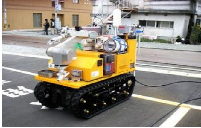
14.109 Monirobo measures radiation following nuclear crisis at Japan's Fukushima Daiichi power plant. http://www.engadget.com/2011/03/23/monirobo-measures-radiation-following-nuclear-crisis-at-japans/
