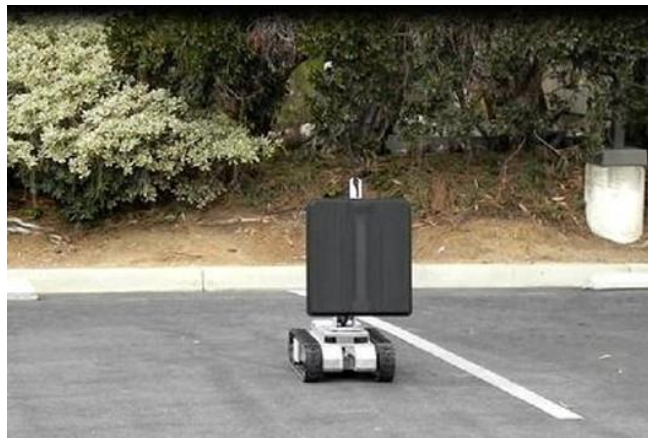
14.23 Cougar20-H surveillance robot that sees through walls and detects breathing, http://www.gizmag.com/cougar20-h-surveillance-robot/17800/picture/129773/
