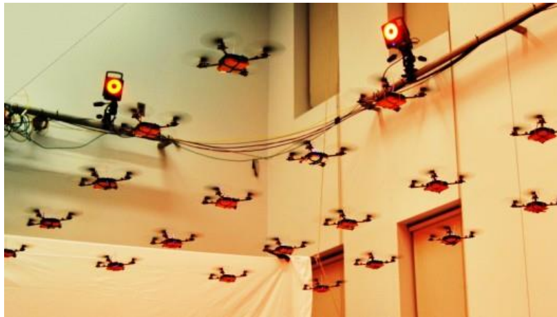
14.199 The autonomous squadron made up of 20 quadrotor robots from KMeI Robotics (Photo: KMeI Robotics) http://www.gizmag.com/grasp-nano-quadrotor-robots-swarm/21302/
