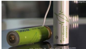
14.81 Brother's AA-size Vibration Energy Cell battery prototype whose generator and rechargeable battery are installed in two different cases. http://www.gizmag.com/brother-vibration-energy-cell-batteries/15804/
