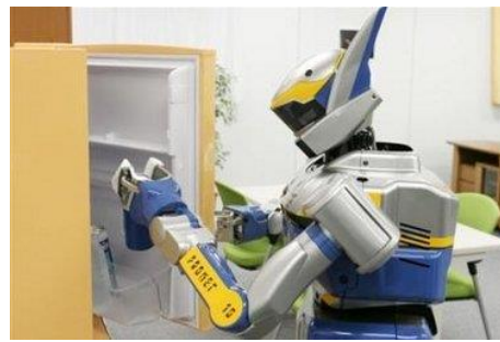
14.17b The HRP-2 completes task such as controlling your TV, moving a chair for you or opening your fridge and getting you a beer by just saying a few voice commands. To see a video of this robot in action. http://hight3ch.com/hrp-2-beer-fetching-bo/
