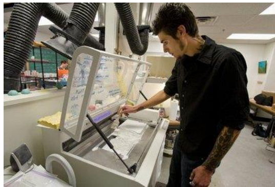
14.54 University of Washington. Grant Marchelli, a UW mechanical engineering graduate student, removes a new object from the Solheim Lab printer. Marchelli led development of the first method for 3-D printing in glass. Reproduced with thanks from, http://www.washington.edu/news/2009/09/24/uw-lab-demonstrates-3-d-printing-in-glass/
