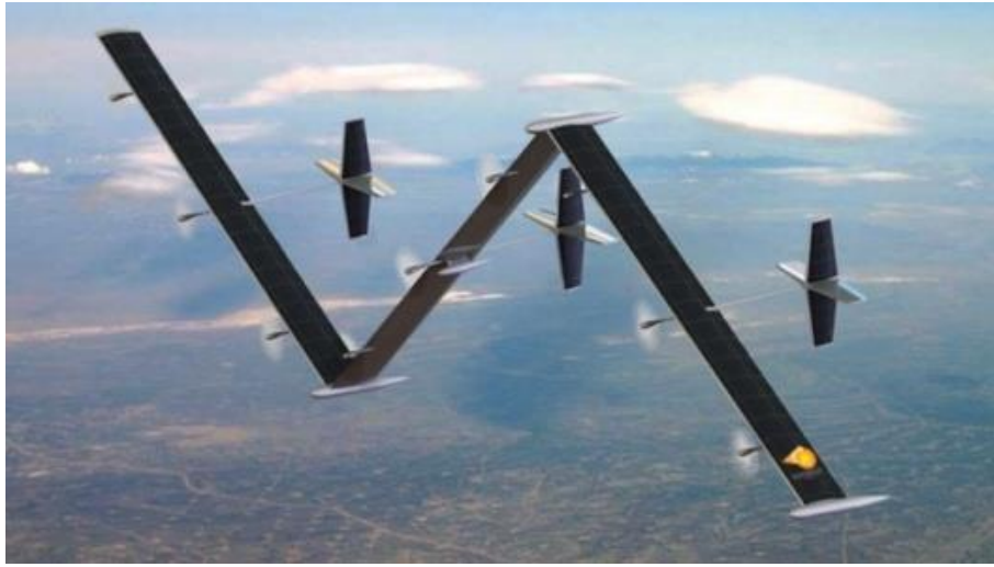
14.30 Odysseus' radical Z-wing configuration. Odysseus: Aurora's radical, unlimited endurance, solar powered aircraft. http://www.gizmag.com/auroras-radical-odysseus-solar-powered-aircraft-unveiled/9261/
